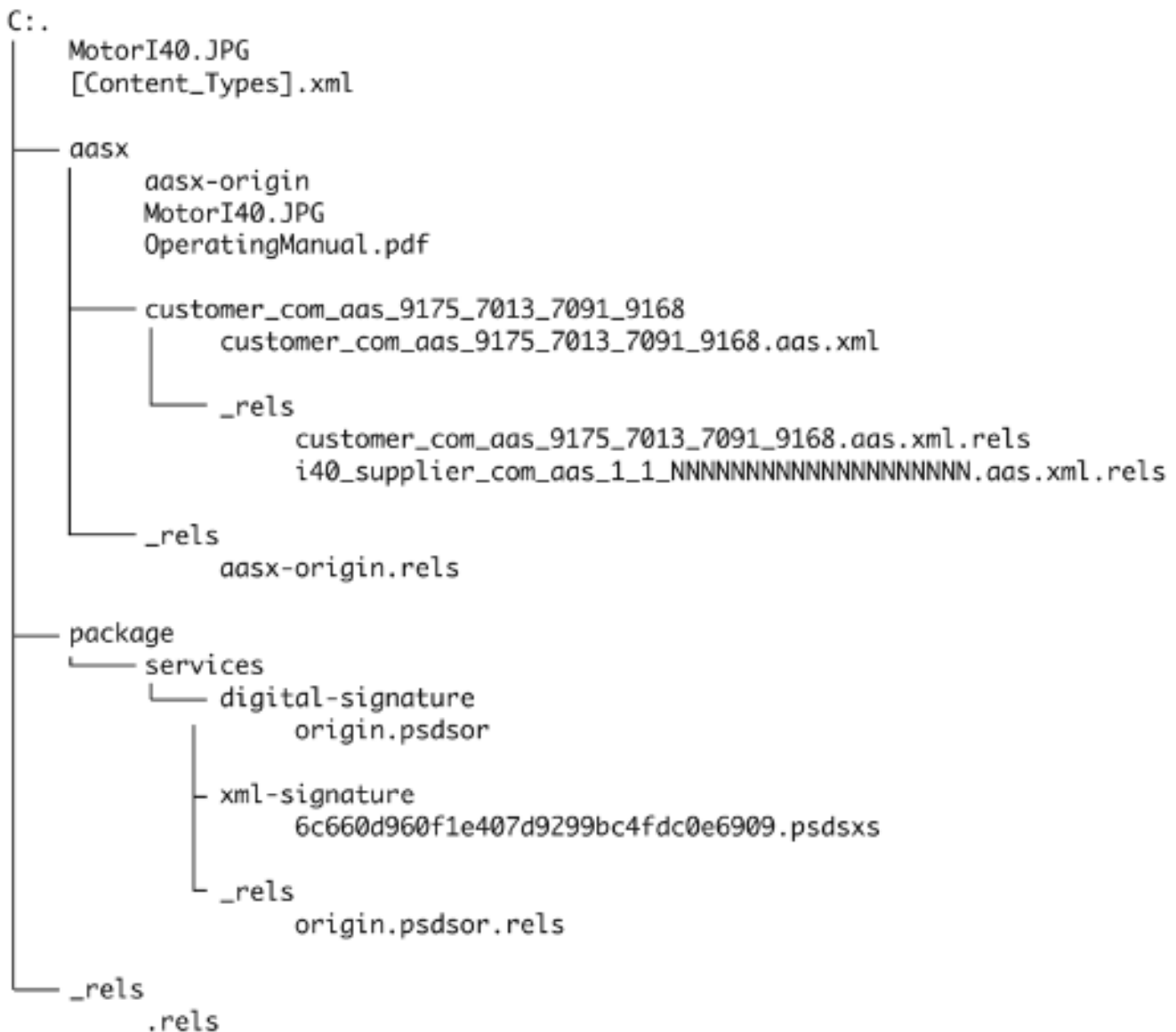
Figure 1: XML-Signature in AAS Structure [8].
