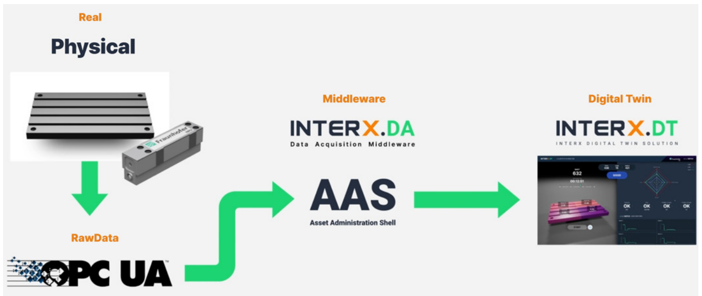
Figure 3 A flowchart of how IIoT and machine data are gathered through AAS and how other AI or Digital Twin solutions are using AAS-gathered data.
